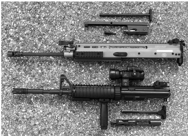
Figure 4.66 (See color insert.) A contrast between the upper receivers of the FN SCAR 16S (top) and an AR-15 (bottom). The bolt carrier groups have been removed to contrast the differences between the two. The SCAR is operated by gas piston; the AR uses the traditional gas impingement. Installed on the AR upper receiver is a Knight's Armament RAS free-floating rail system, an aftermarket flash hider, a MaTech rear sight, a Knight's Armament vertical fore grip, and an Aimpoint Comp M4 using a Knight's Armament mount. (Image from author's collection.)
